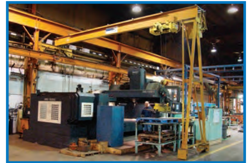
A 3-Ton Spanco Single Leg Gantry Crane with one end supported on the wall and one end traveling along the floor.
