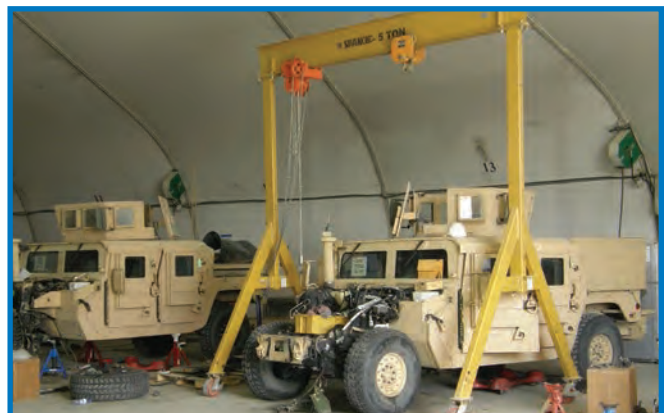
Spanco 5-ton A Series Gantry Crane lifting engines from military vehicles for maintenance.
