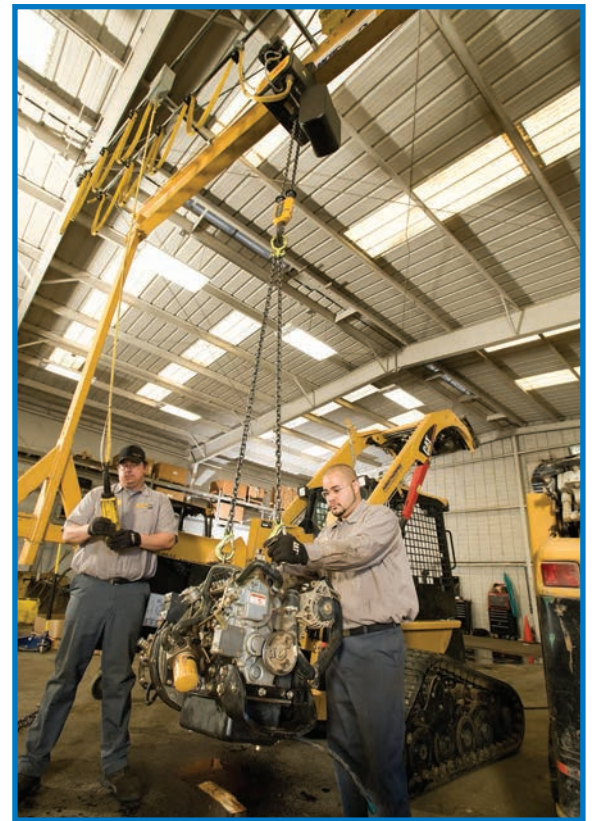
A Series Gantry Crane lifting an engine from a small loader.
